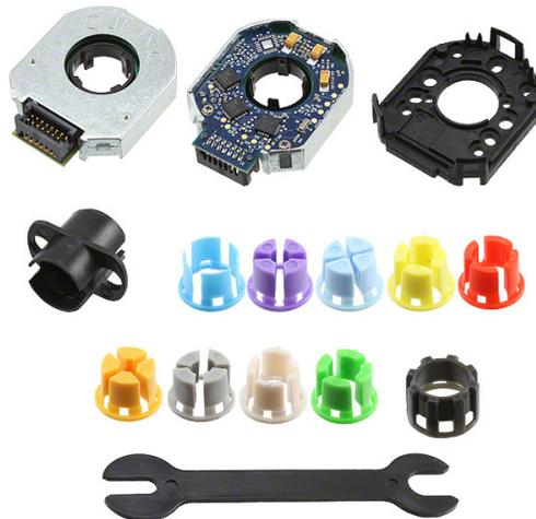
**MA3** magnetic encoder that comes in 10 bit and 12 bit version (10bit has 1kHz refresh rate, 12bit has 244Hz refresh rate). <http://www.usdigital.com/products/encoders/absolute/rotary/shaft/MA3>
