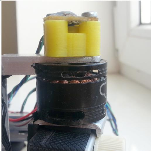
AMT203 encoder has pass-through hole and comes fully assembled with variety set of shaft adapters and centering tool. You only need to make cabling (cable and connector not included)
